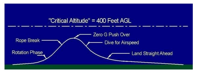
If the nose is up 45 degrees at the failure, the glider will be losing airspeed at about 12 knots per second, so the pilot must react swiftly. The correct response is to push over vigorously in a zero G ballistic trajectory. **Do not delay the recovery.**
