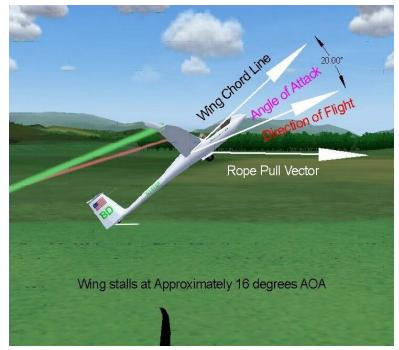
amount of yaw (rudder input) and maintain a shallow climb until adequate speed is seen with continuing acceleration. Consider adequate speed to be 1.5 times the stall speed. Also ensure the transition from initial lift off to full climb is controlled and progressive. The pilot should be trying to achieve a smooth rotation with airspeed increasing to a stable climb speed as one would do with a high performance airplane.
