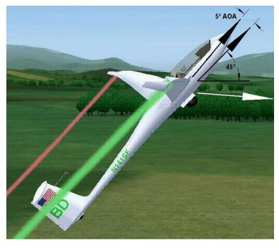
so there is little tension on the rope. Cutting power will increase the sag of the rope so the automatic release is triggered. The pilot will pull the release anyway to assure rope separation.
